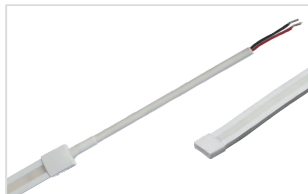
4 Install end cap Insert the end cap into the wire. Inject the glue into the end cap, and slipped the end cap, clean the excess glue.
